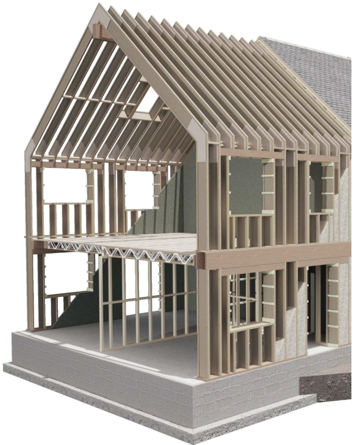
Figure 7: Cutaway Illustration of the Common House using the PH15 system by PH Homes. The system efficiently uses engineered timber portal frame to reduce material waste, while providing a wide cavity to super-insulate the frame.
